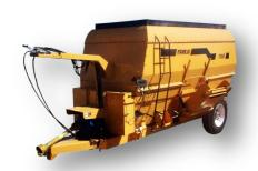
The mixer has a control lever located on the goose to activate the download and distribution of feed in the hopper, you must maneuver a lever to open the door, another to activate the band when you go to deposit the mix in the forage feeders and another to lower or raise the band.
